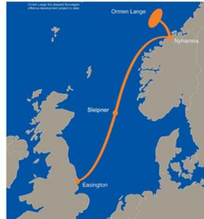
But Ormen Lange is not easy to exploit. The gas field itself lies roughly 3000 meters below sea level, buried beneath an uneven seabed and sitting under 800 to 1100 meters of water. Situated 120 km off the coast of Norway, the site experiences some extreme natural conditions. There are subzero temperatures, whether measured in Fahrenheit or Centigrade, most of the year. The seas are stormy, with strong underwater currents.
