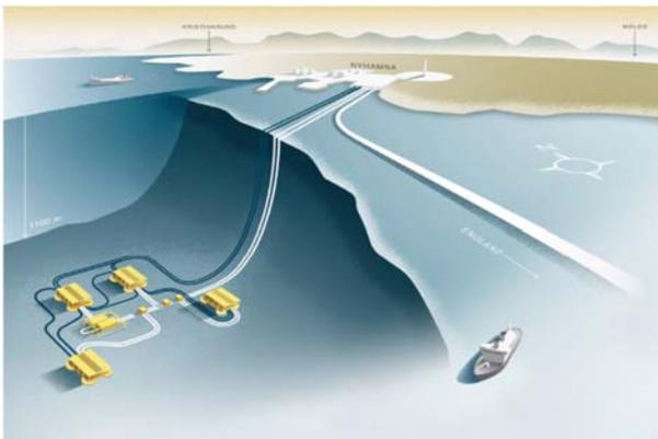
As for project itself, it consists of a 24 subsea wells in four seabed templates. The output of the wells is sent in pipes 120 km to Nyhamna on the island of Aukra on the west coast of Norway. There the fuel is processed and readied for shipment to the U.K. via a 1200 km long undersea pipeline.
