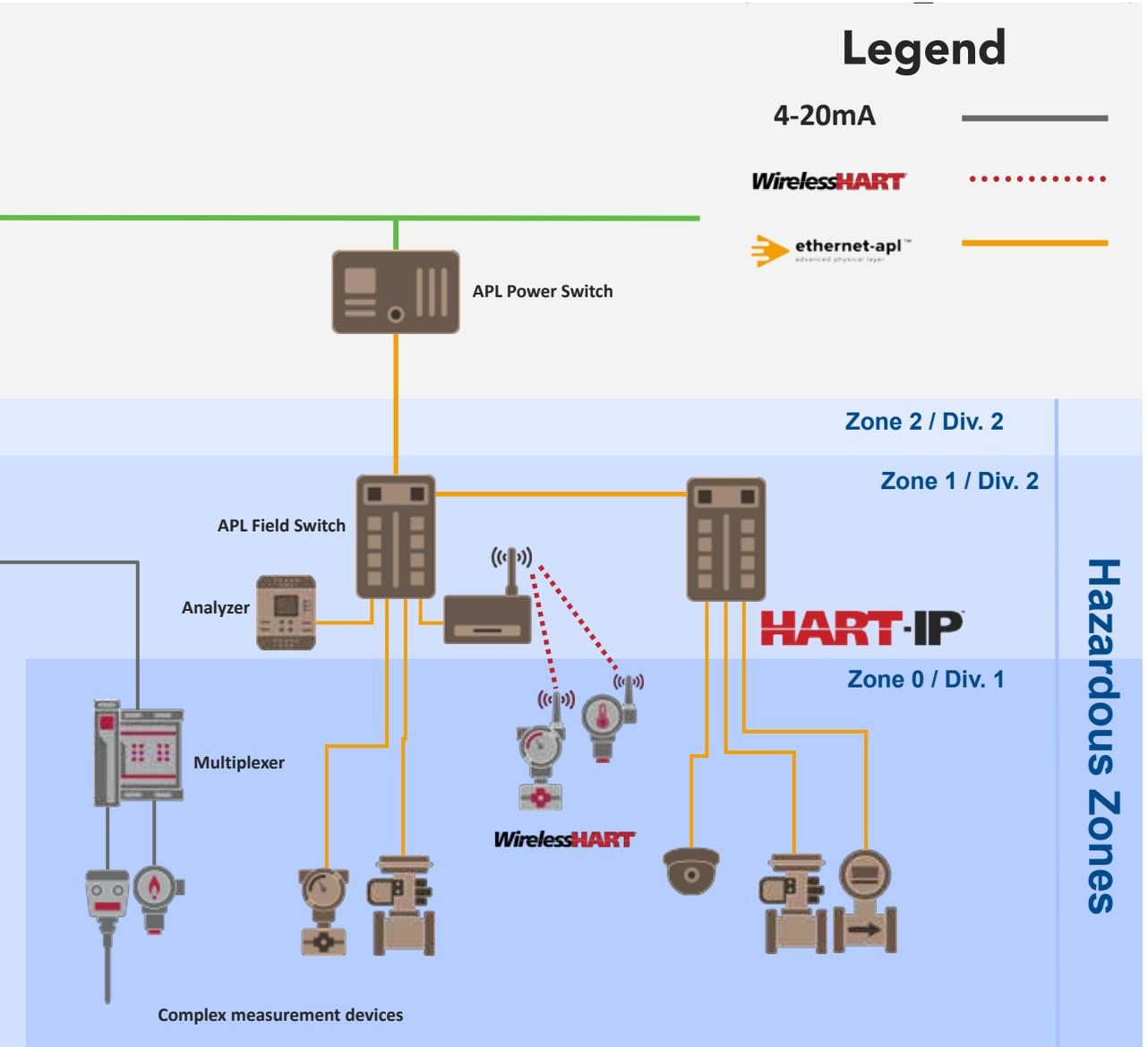
control network. As Ethernet-APL instruments become available, they can be connected to the area control network via HART-IP (orange connections) through a simple APL field switch. And as confidence grows, an APL
