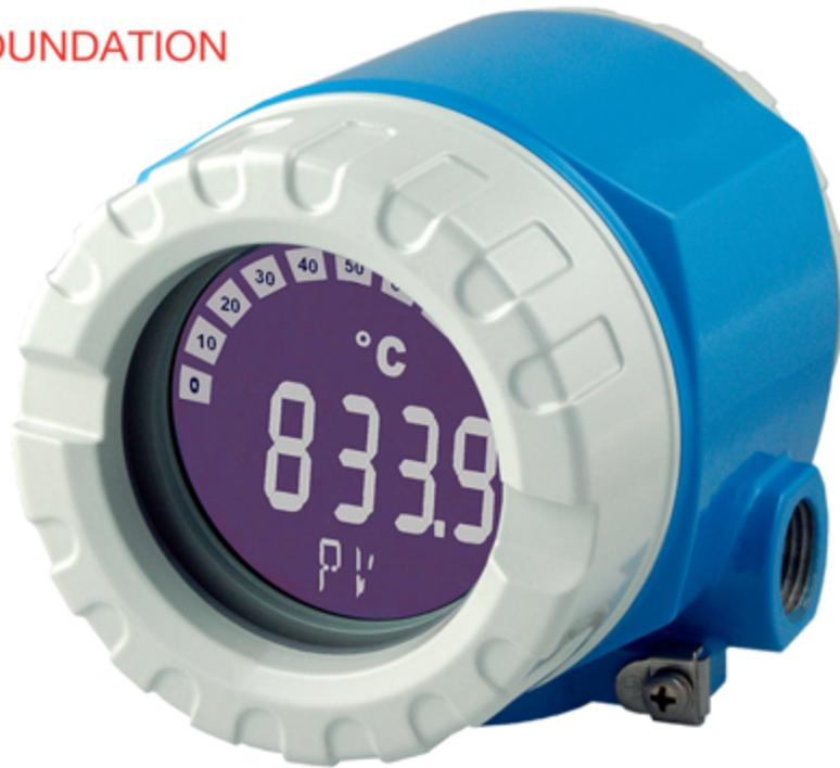
The iTEMP TMT162 transmitter supports two-channel operation with monitoring of redundancy and temperature drift, as well as calculation of differential and average temperature. In order to ensure highest accuracy in critical applications, sensors can be matched by Callendar/Van Dusen equation or linearization.
