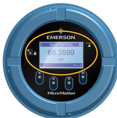
The LCD panel also provides access to the display menus and alert information. From the display menus, you can:
