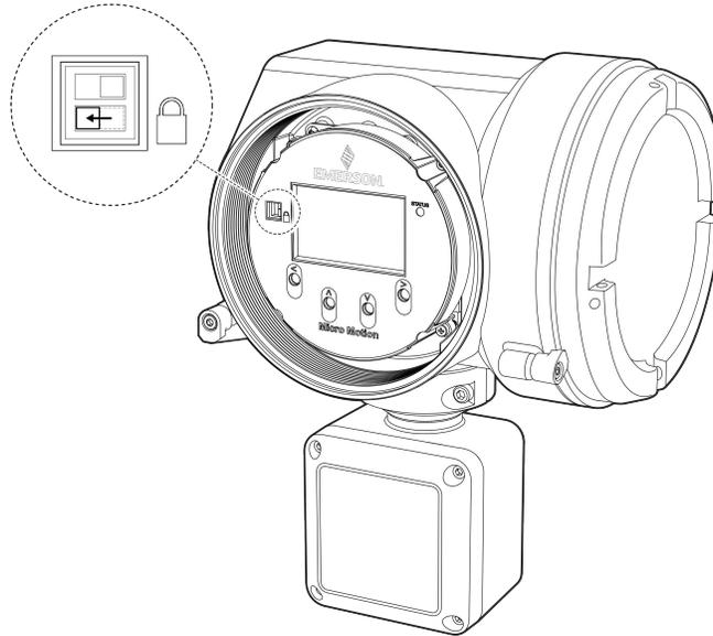
You can determine whether you need to lock or unlock the transmitter by looking at the switch.
