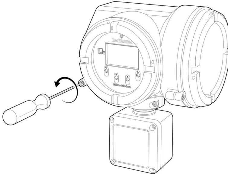
3. Using a fine-pointed tool, move the switch to the desired position.
