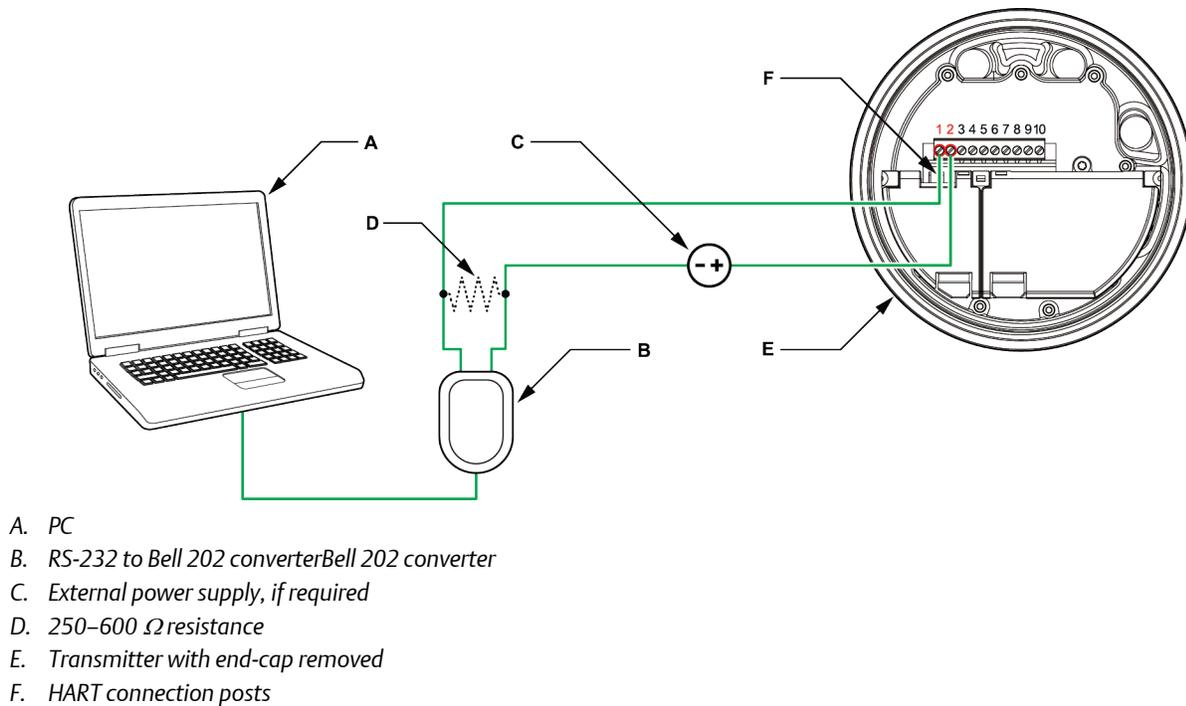
The signal converter must be connected across a resistance of 250–600  $\Omega$ . The mA output requires an external power supply with a minimum of 250  $\Omega$  and 8 V. See the following figure to help determine the appropriate combination of voltage and resistance. Note that many PLCs have a built-in 250- $\Omega$  resistor. If the PLC is powering the circuit, be sure to take this into consideration.
