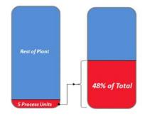
8% of the Process Units accounted for 48% of the Instrument Downtime (hrs)
